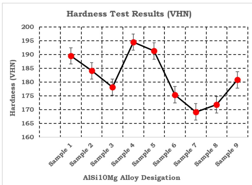
**Figure 2: Hardness Test Results of AlSi10Mg**
