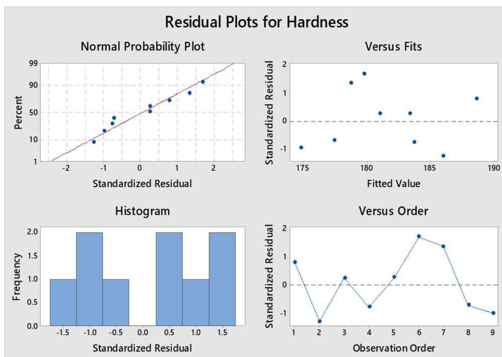
**Figure 4: Normal Probability and Residual Plots of Hardness for all combinations considered**
