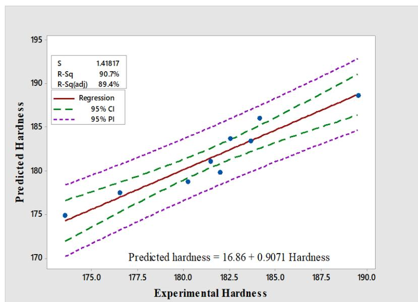
**Figure 3: Predicted and Experimental Hardness for all combinations of AlSi10Mg**
