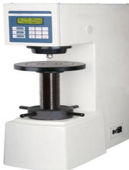
Figure 1: Hardness Tester [10].
