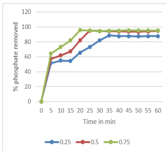
**Fig:4 effect of contact time on chemically activated carbon  $\text{CaCl}_2$**
