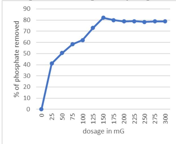
**Fig:5 effect of optimum dosage on physically activated carbon**
