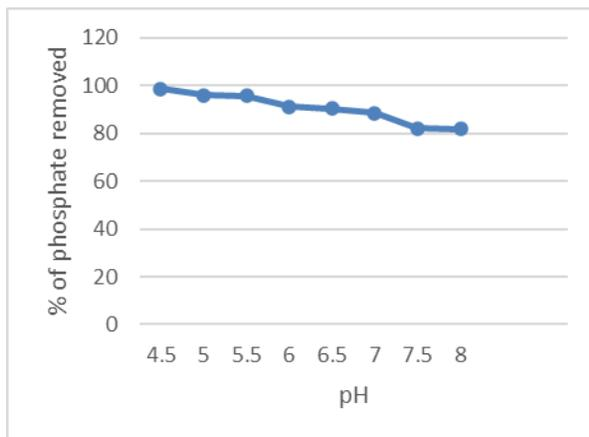
**Fig:7 effect of pH on physically activated carbon**
