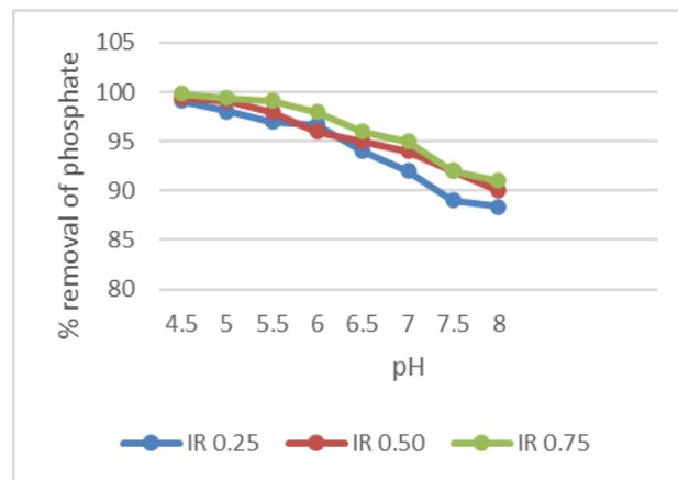
**Fig:8 effect of pH on chemically activated carbon CaCl<sub>2</sub>**
