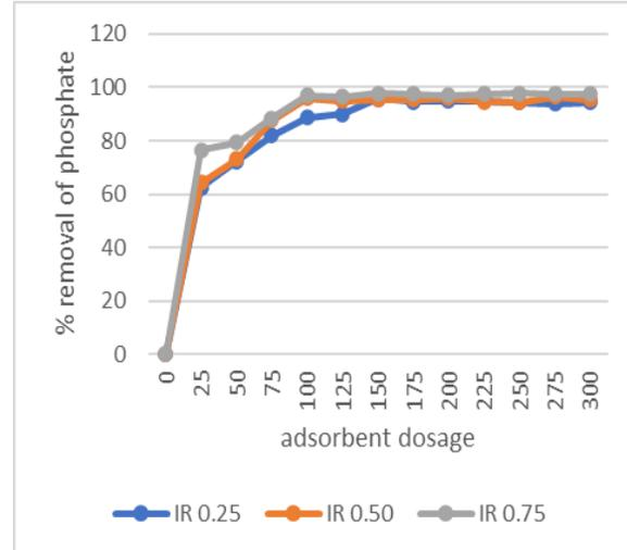
**Fig:6 effect of optimum dosage on chemically activated carbon CaCl<sub>2</sub>**
