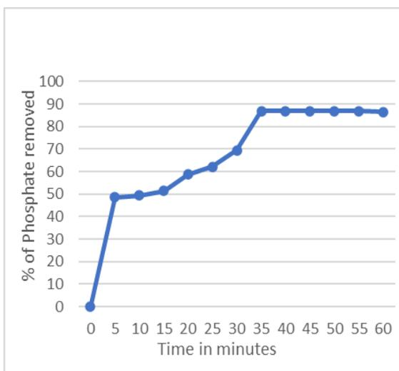
**Fig:3 effect of contact time on physically activated carbon**
