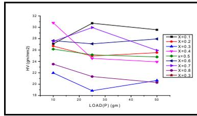
Figure 7: Micro hardness of  $(\text{KCl})_{0.9-x}(\text{KBr})_x(\text{NaI})_{0.1}(\text{Li}_2\text{SO}_4)_{0.05}$  crystals grown by Evaporation method
