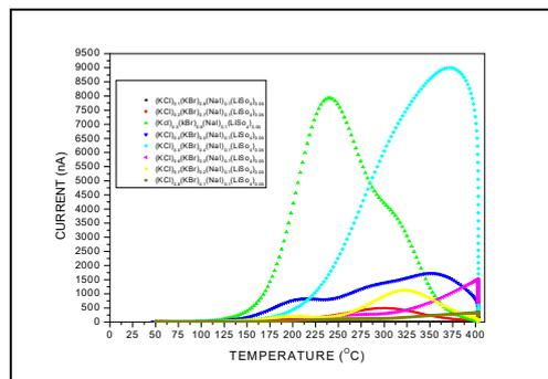
Figure3. Thermo luminescence glow curve of  $(\text{KCl})_{0.9-x}(\text{KBr})_x(\text{NaI})_{0.1}$  ternary crystal doped with  $(\text{Li}_2\text{SO}_4)_{0.05}$  grown by Melt method irradiated with a dosage of 15Mrad.
