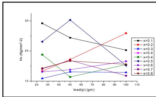
Figure 8: Micro hardness of  $(\text{KCl})_{0.9-x}(\text{KBr})_x(\text{NaI})_{0.1}(\text{Li}_2\text{SO}_4)_{0.05}$  crystals grown by Melt method
