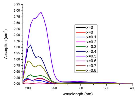
Figure 6: Optical absorption of  $(\text{KCl})_{0.9-x}(\text{KBr})_x(\text{NaI})_{0.1}(\text{Li}_2\text{So}_4)_{0.05}$  Crystal Grown by Evaporation method irradiated with a dosage of 15Mrad.
