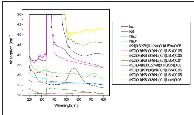
Figure.5. Optical Absorption Spectra of KCl, KBr, NaCl, NaBr,  $(\text{KCl})_{0.9-x}(\text{KBr})_x(\text{NaI})_{0.1}$  ternary crystal doped with  $(\text{LiSo}_4)_{0.05}$  grown by melt method irradiated with a dosage of 15 Mrad.
