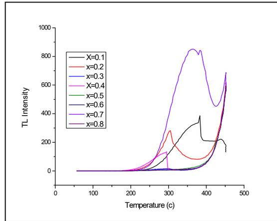
Figure4. Thermo luminescence glow curve of  $(\text{KCl})_{0.9-x}(\text{KBr})_x(\text{NaI})_{0.1}$  ternary crystal doped with  $(\text{LiSo}_4)_{0.05}$  grown by Evaporation method irradiated with a dosage of 15Mrad.
