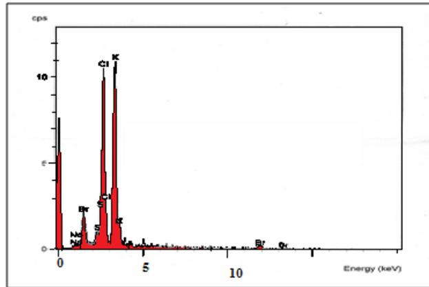
Figure 1. EDAX report of  $(\text{KCl})_{0.8}(\text{KBr})_{0.1}(\text{NaI})_{0.1}(\text{Li}_2\text{SO}_4)_{0.05}$  crystal grown by Evaporation method.
