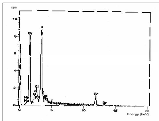
Figure 2. EDAX report of  $(\text{KCl})_{0.1}(\text{KBr})_{0.7}(\text{NaI})_{0.1}(\text{Li}_2\text{SO}_4)_{0.05}$  crystal grown by Melt method.
