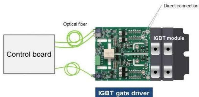
Figure 5.Connection from Control Card
