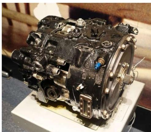
**Figure 1. Integrated Drive Generator**
