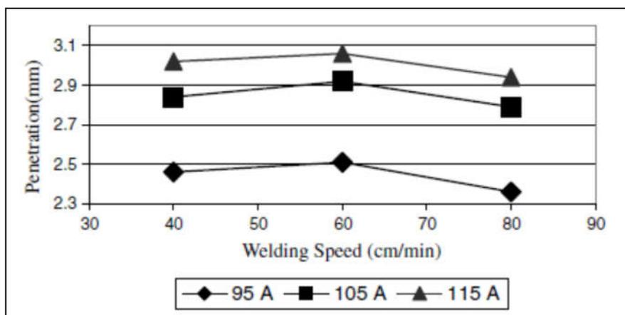
Figure 1: *Penetration vs. Welding speed diagram for 22 V constant arc voltages.*
