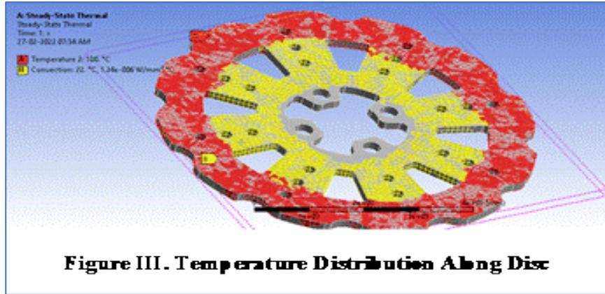
Figure III. Temperature Distribution Along Disc
