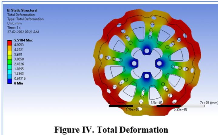
Figure IV. Total Deformation
