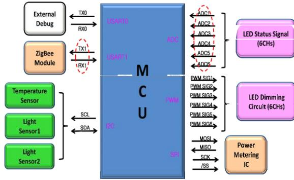
Fig.4. MCU Communication Block Diagram
