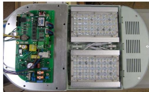
Fig.7. Smart LED Light Panel using ZigBee Protocol
