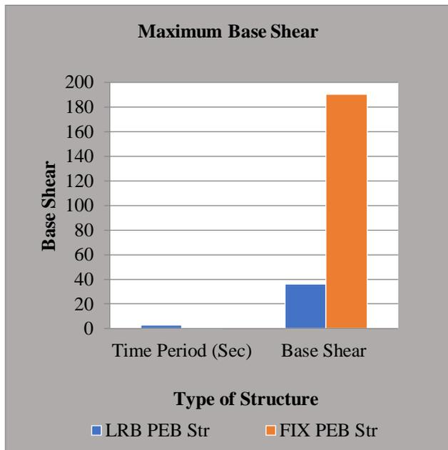
**Figure-4.1: Maximum Base Shear**
