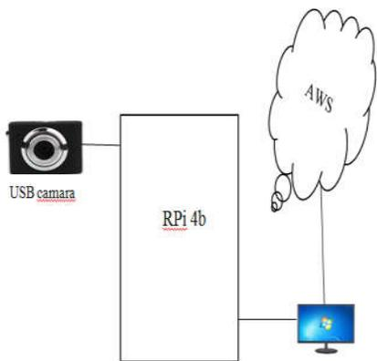
Figure 1 Plant Disease Detection System
