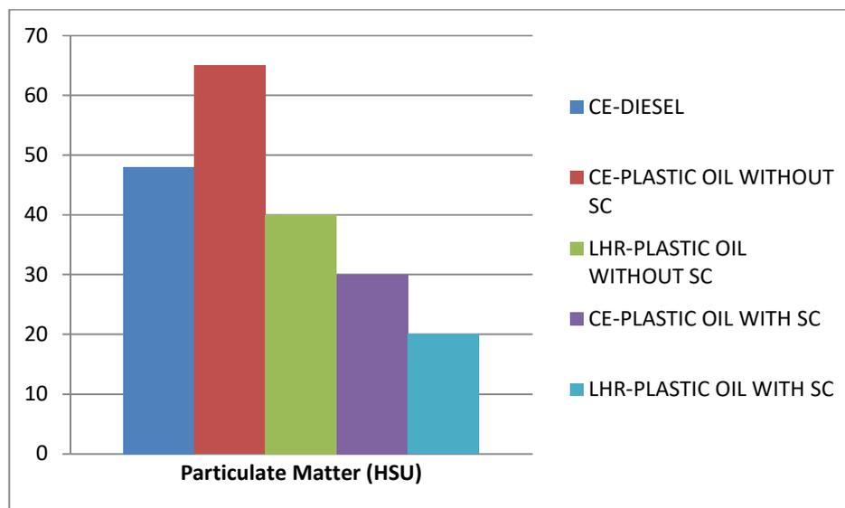
**Fig.3. Variation of particulate matter at full load**
