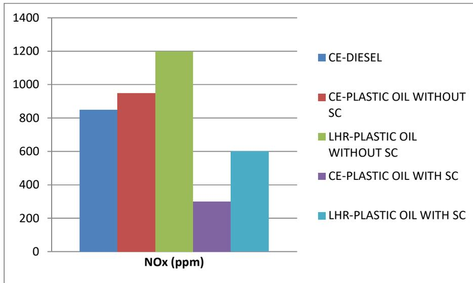
**Fig.6 Variation of NO<sub>x</sub> levels at full load**
