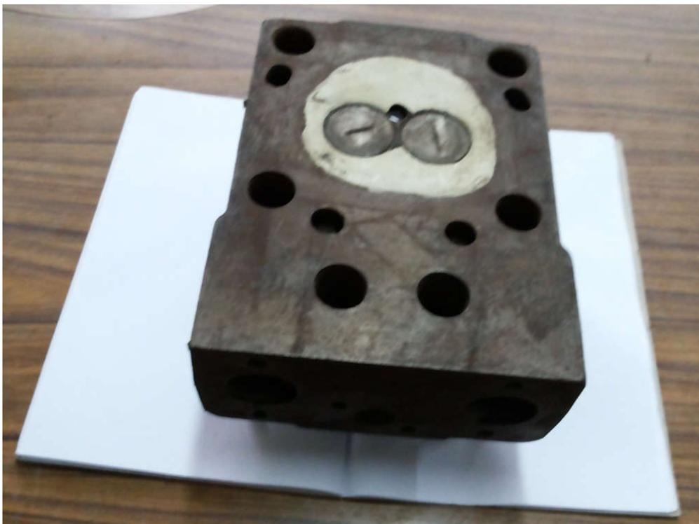
Fig.1. Photographic view of ceramic coated cylinder head
