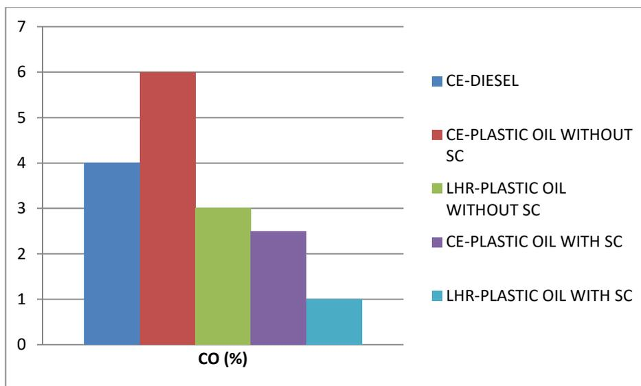
**Fig.5 Variation of CO levels at full load**
