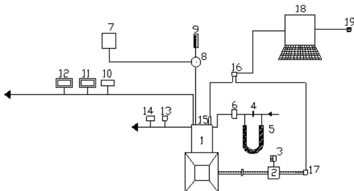
1.Engine, 2.Electical Dynamometer, 3.Load Box, 4.Orifice meter, 5.U-tube water manometer, 6.Air box, 7.Diesel tank, 8 Three-way valve, 9.Burette, 10. Exhaust gas temperature indicator, 11.AVL Smoke meter, 12.Multi Gas Analyzer, 13.Outlet jacket water temperature indicator, 14. Outlet-jacket water flow meter, 15.Piezo-electric pressure transducer, 16.Console, 17.TDC encoder, 18.Personal Computer and 19.Printer.
