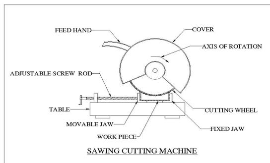
**Fig. 3.2** Sawing Cutting Machine
