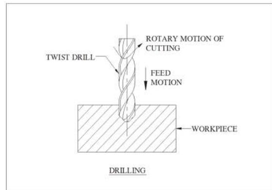
**Fig. 3.4** Drilling Process
