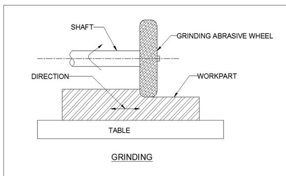
**Fig. 3.5** Grinding Process
