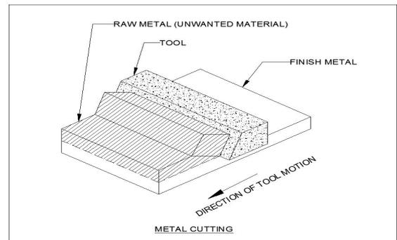
**Fig.3.1** Metal cutting process
