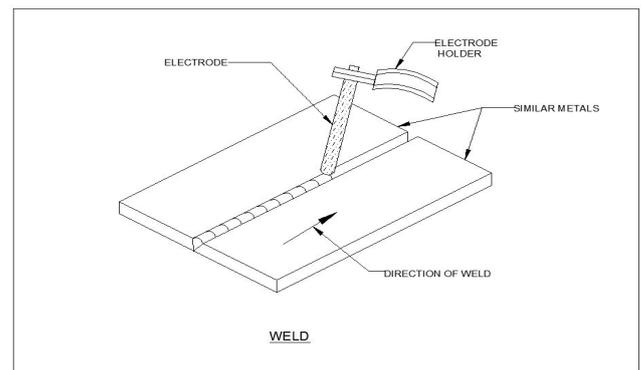
**Fig. 3.3** Welding Process
