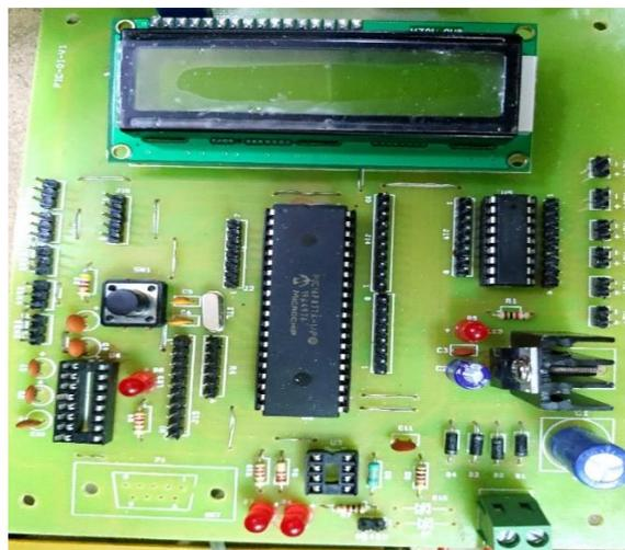
**FIG 4. PIC (16F877A) Microcontroller Board**
