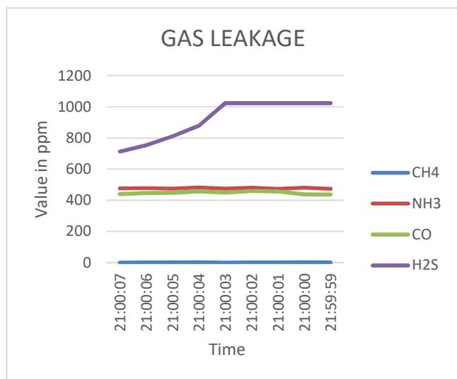
Fig 3. Comparison of Gas Leakage detection with respect to Time (second) for table 1
