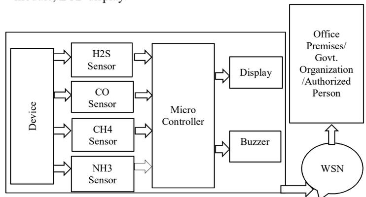
Fig 1. Block diagram of WSN-Based Gas Leakage Detection System
