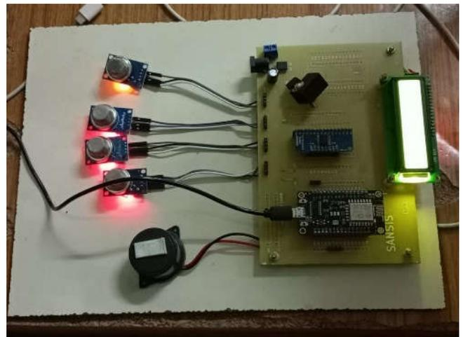
Fig 2. Implementation of Gas Leakage detection system
