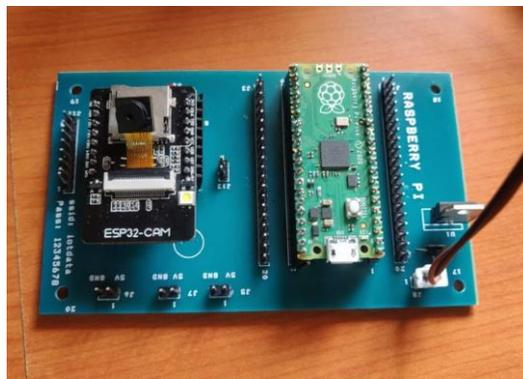
**Figure 1.** ESP32 CAM with Raspberry Pi Pico Module
