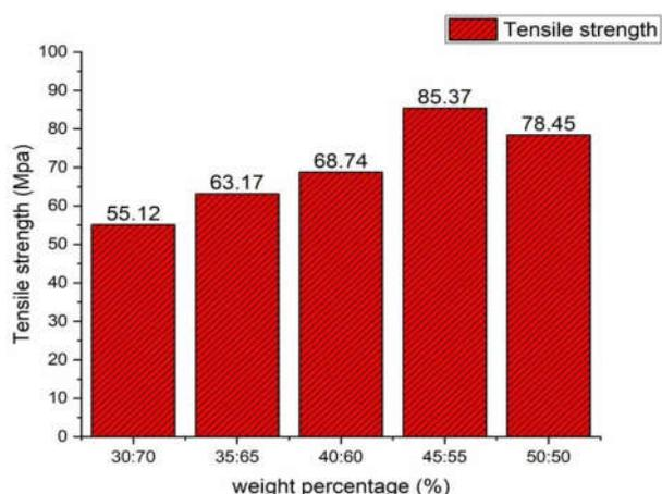
Fig. 3.1 Tensile strength of cotton & bamboo epoxy composite
