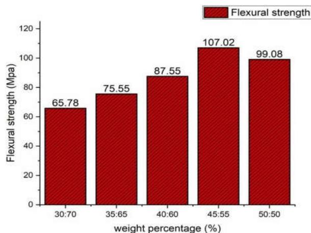
Fig. 3.2 Flexural strength of cotton & bamboo epoxy composite
