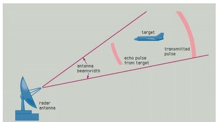
Fig (a) Principle of Radar Operation
