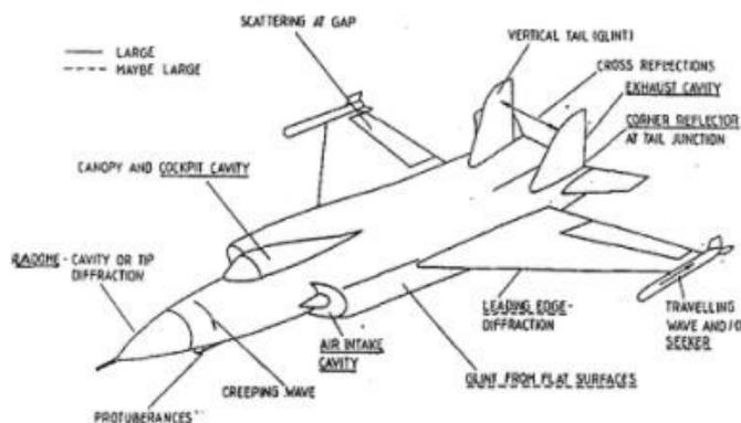
Fig (e) Contribution to the radar cross section
