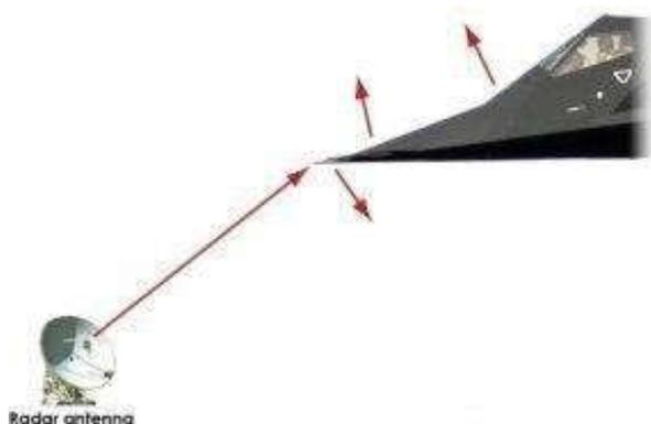
Fig (c) Scattering of radar waves
