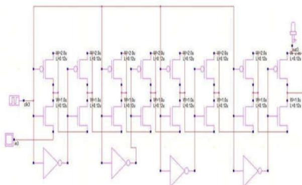
Fig 6: Serial In-Serial Out shift register
