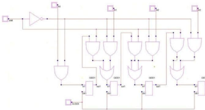
Fig 8: Parallel In-Serial Out shift register
