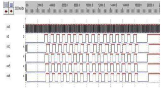
Figure11: Simulation output of SIPO
