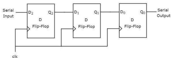
Fig 1: Serial In – Serial Out shift register
