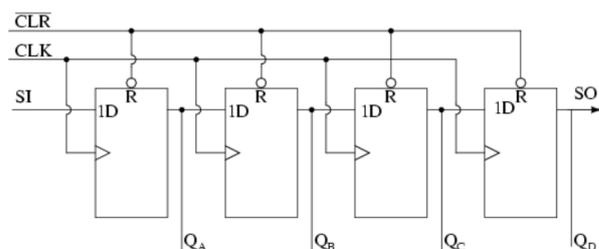
Fig 2: Serial In-Parallel Out shift register
