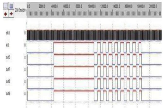
Figure13: Simulation output of PIPO
