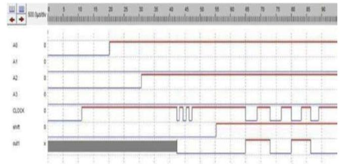
Fig 12: Simulation output of PISO
