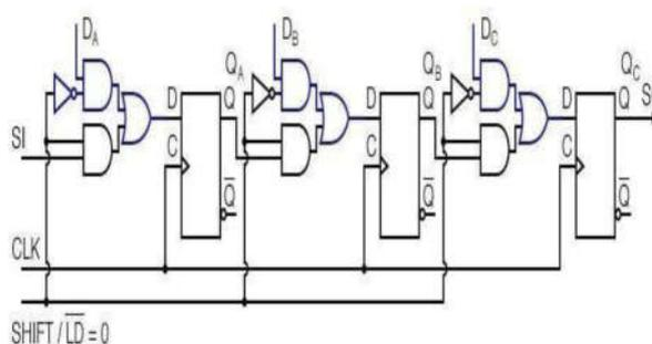
Fig 3: Parallel In - Serial Out shift register
