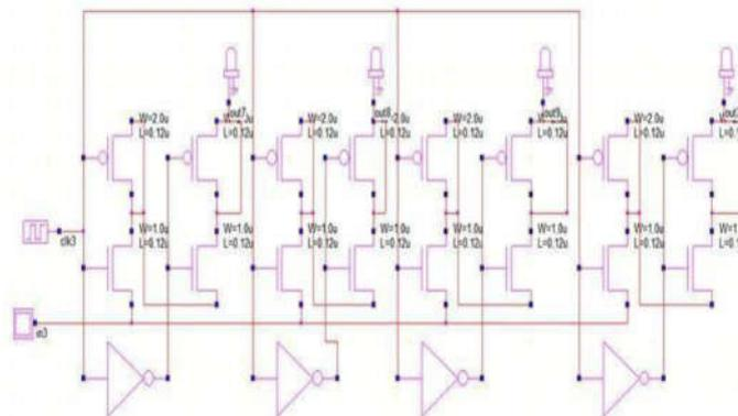
Fig 9: Parallel In-Parallel Out shift register
