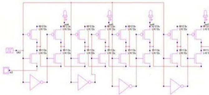
Fig 7: Serial In-Parallel Out shift register
