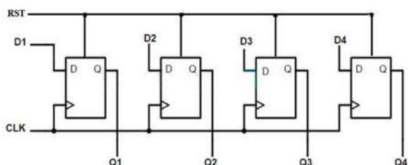
Fig 4: Parallel In - Parallel Out shift register
