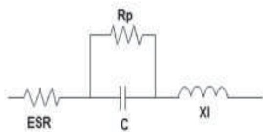
Fig 2- Equivalent simplified model of supercapacitor
