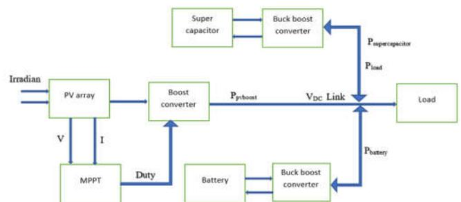
Fig 6-Schematic block diagram of proposed work.
