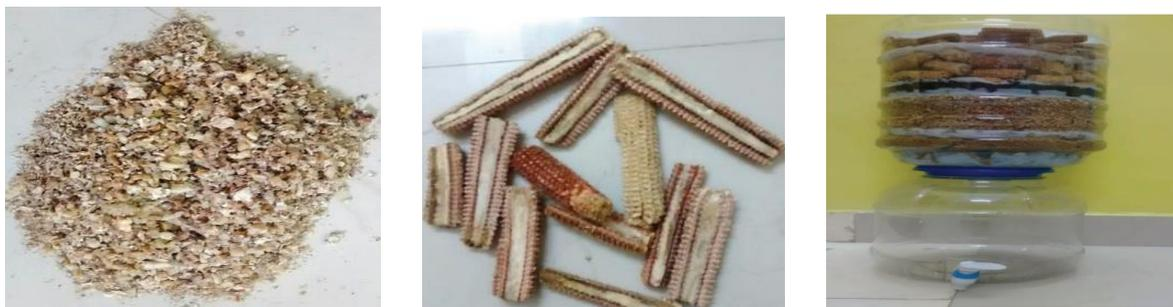
**Figure 1. Images of the filter with biomass materials used to filter grey water from kitchen waste.**
