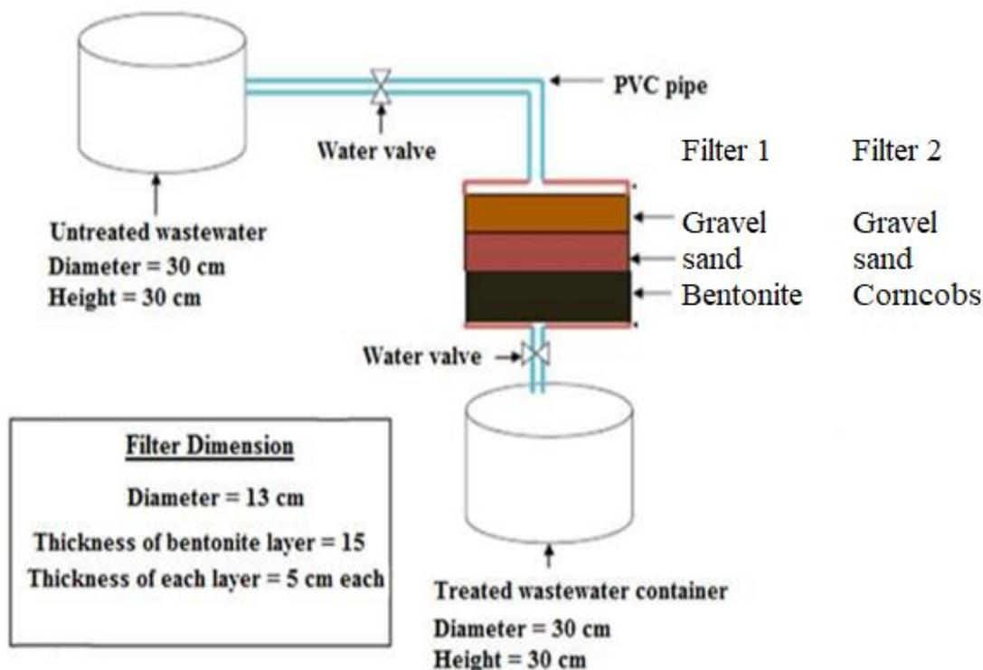
Figure 5. Illustration of filter 1 using bentonite and filter 2 using corncobs.
