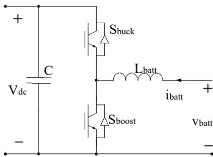
Fig. 2. Battery charger design
