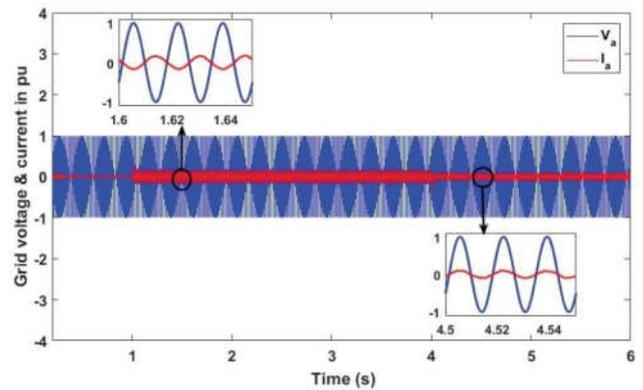
Fig 9. During V2G-Operation grid voltage and grid injected current
