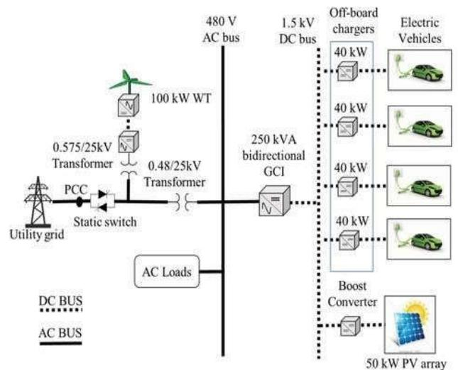
Fig 6. Proposed microgrid test system configuration.
