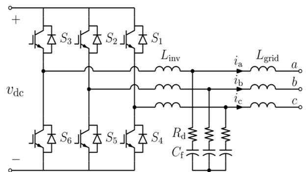
Fig 3. Three phase inverters plus LCL filter
