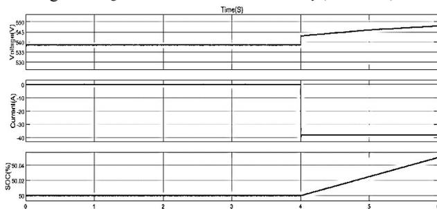
Fig 8. Voltage, Current and SOC of EV2 battery (G2V mode)
