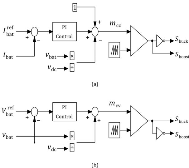
Fig 3,(a),(b). Constant current and voltage control methods for battery charge.
