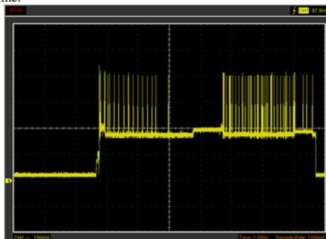
**Figure 4. Oscillogram of voltage across current sensing resistor of 2.7 Ω set at 1s per Division**
