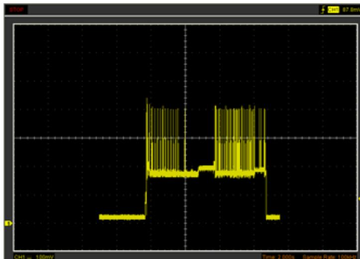
**Figure 3. Oscillogram of voltage across current sensing resistor of 2.7 Ω in Deep sleep mode operation of NodeMcu**
