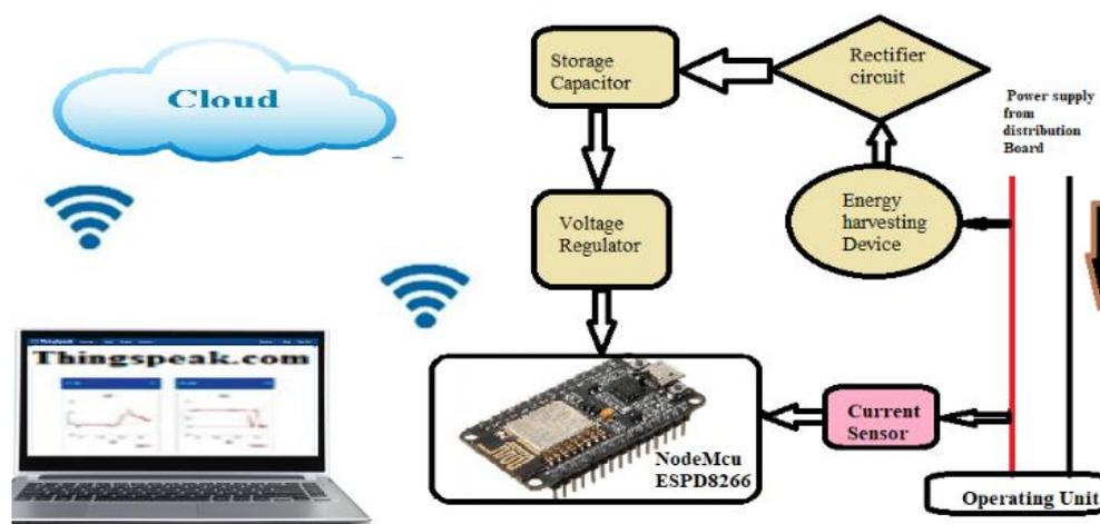
**Figure 1. Arrangement of component required for monitoring based on IoT in connection with Energy harvesting systems.**
