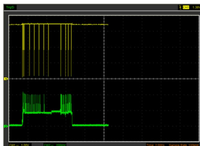
Figure 5. Waveforms from sensing resistor and TX pin of NodeMcu.
