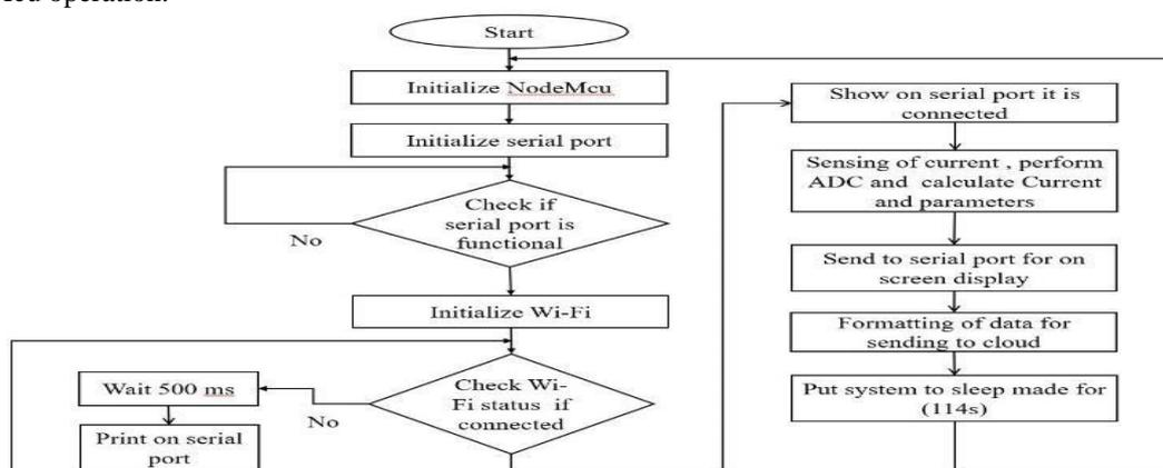
Figure 2. Process flow chart of NodeMcu
