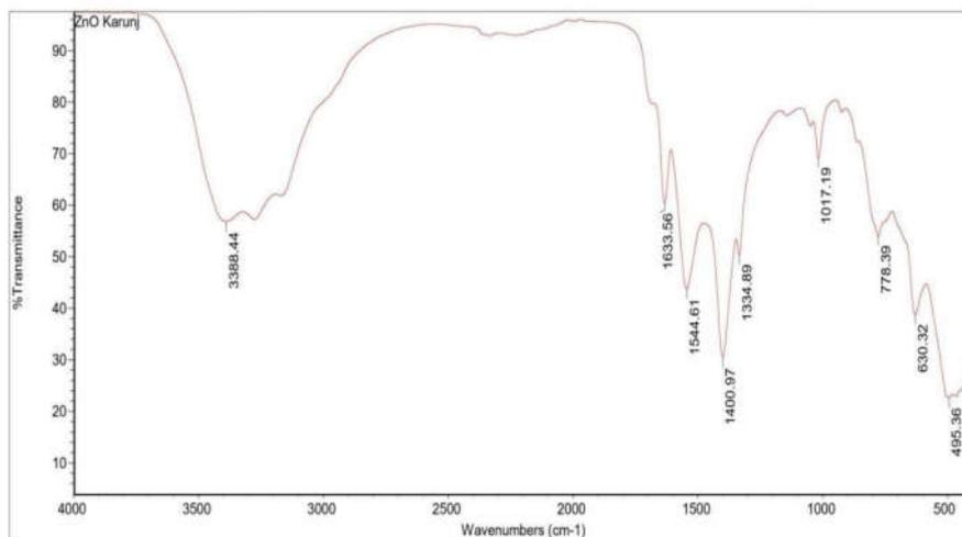
**Figure. 2: FTIR spectrum of ZnO nanoparticles**
