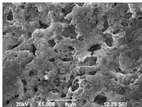
**Figure No.7: SEM Image of ZnO Nano Particles with magnification of x 5000**
