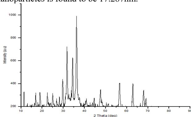
Figure.1: Powder XRD pattern of ZnO nanoparticles
