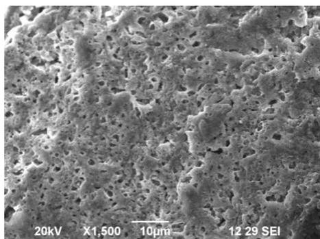
**Figure No. 6: SEM Image of ZnO Nano Particles with magnification of x 1500**
