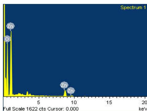
**Figure.5:EDAX Spectrum of ZnO nanoparticles**
