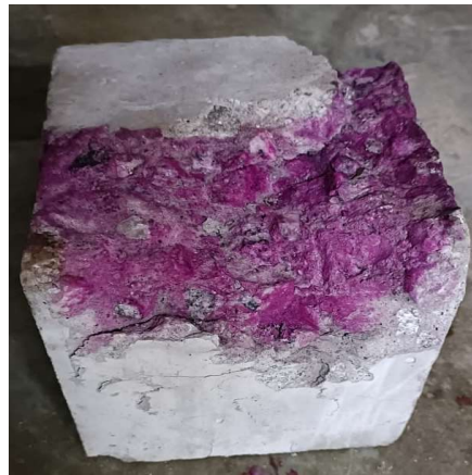
Figure.3 Carbonation Test on Concrete Cube
