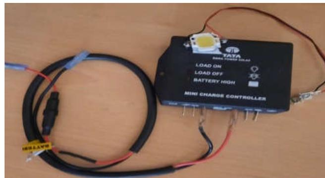
**Figure 5 Solar charge controller**
