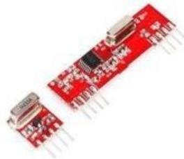
Figure 5. RF module – 433mhz
