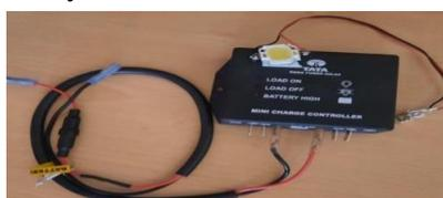
Figure 3. Solar charge controller
