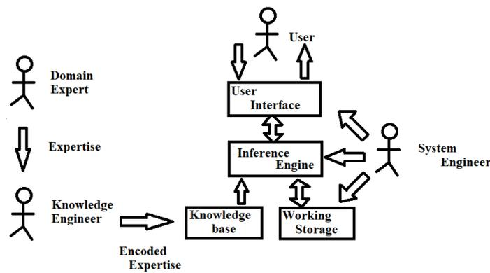
Figure 2. Components of an Expert System
