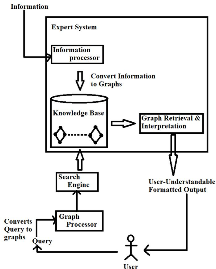
Figure 12. Processing of Graphs in an Expert System
