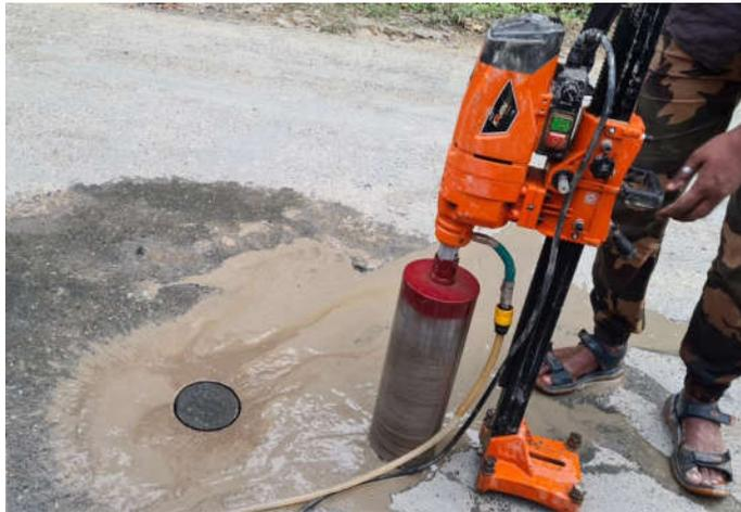
Figure 3: Showing Core Drilling at site for testing
