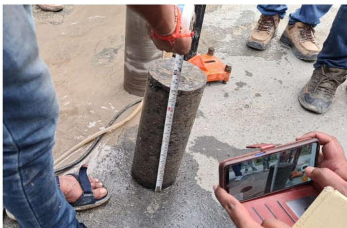
Figure 4: Intact Recovered Core as designed for Lab test
