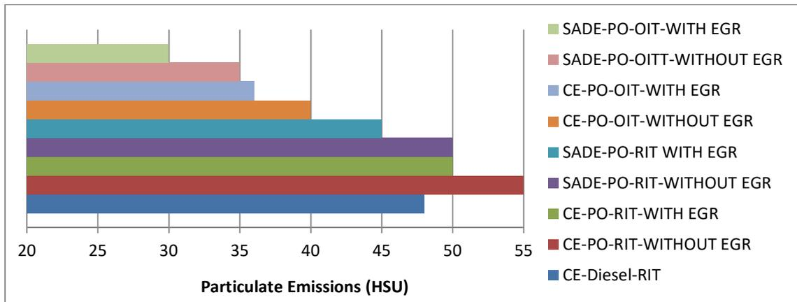
**Fig. 4 Variation of Particulate Emissions, at Full Load .**
