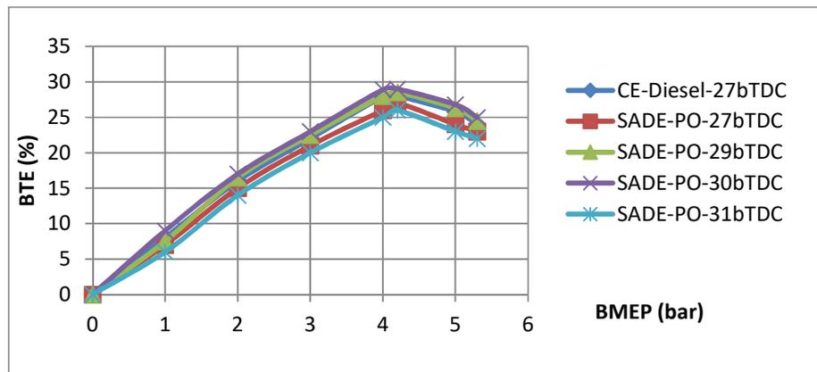
**Fig.3.Variation of BTE with BMEP in SADE with advanced injection timing**
