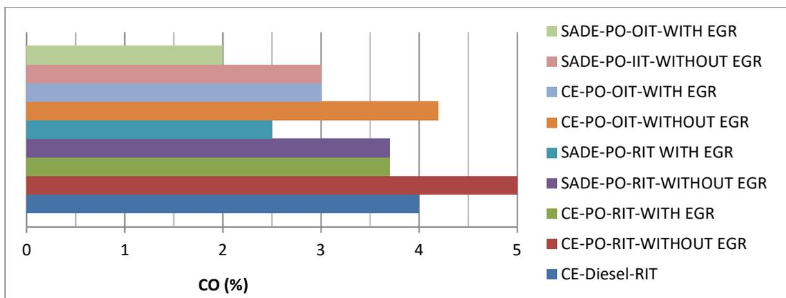
**Fig.5 Variation of CO emissions at full load**
