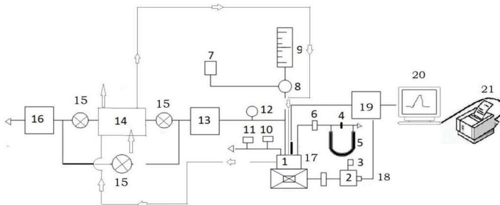
1.Engine, 2.Electical Dynamometer, 3.Load Box, 4.Orifice meter, 5.U-tube water manometer, 6.Air-box, 7.Fuel tank, 8. Pre-heater, 9.Burette, 10.Outlet jacket water temperature indicator, 11. Outlet jacket water flow meter, 12. Exhaust gas temperature indicator, 13. AVL Smoke meter, 14. Heat exchanger(HE), 15.Control valve, 16. Netel Chromatograph NO<sub>x</sub> analyzer 17. Piezo electric pressure transducer, 18.TDC encoder, 19.Console, 20.Personal computer and 21.Printer.
