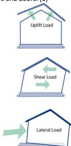
Figure 1.2 Loads acting on structures due to wind loads<sup>4</sup>
