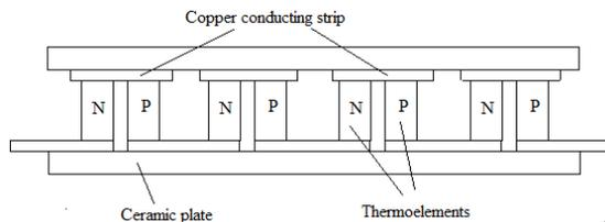
Fig.1 Basic single stage thermoelectric module
