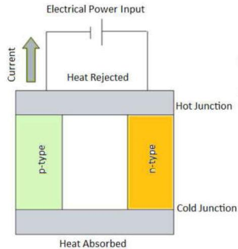
Fig.3 TEM used as refrigerator
