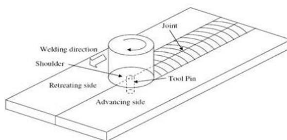
Figure 1: Schematic drawing of friction stir welding [1]
