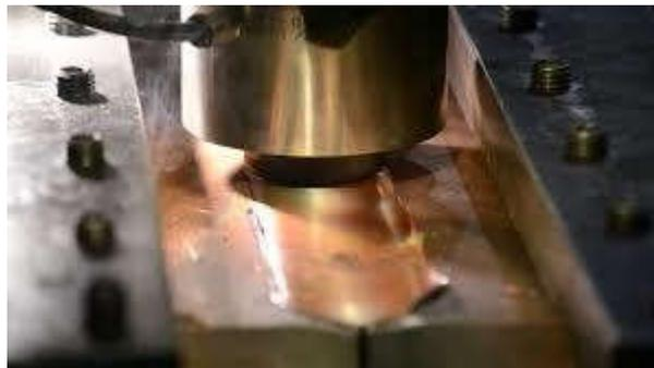
**Figure 2: Welding of Copper by friction stir welding**
