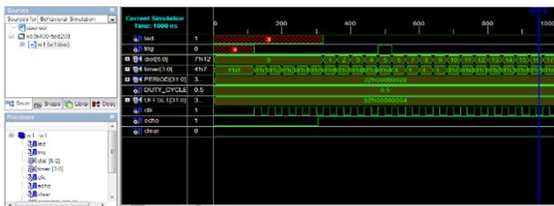
Fig 10: Represents the snapshot of Ultrasonic Sensor Simulation
