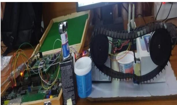
Fig 11. Overview of the model (Smartbin) and Ultrasonic and moisture sensors detecting object and moisture content in object.
