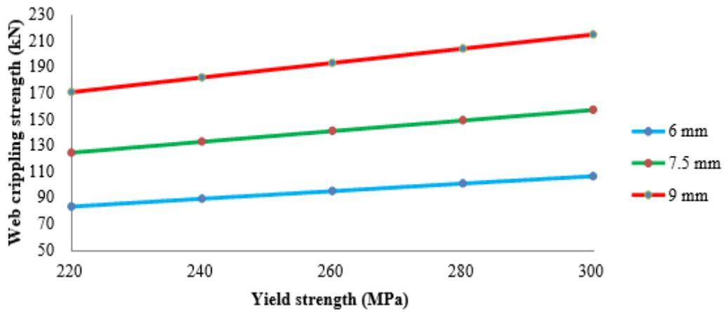
Fig 9. Variation of web crippling strength with yield strength for 130x65 sample
