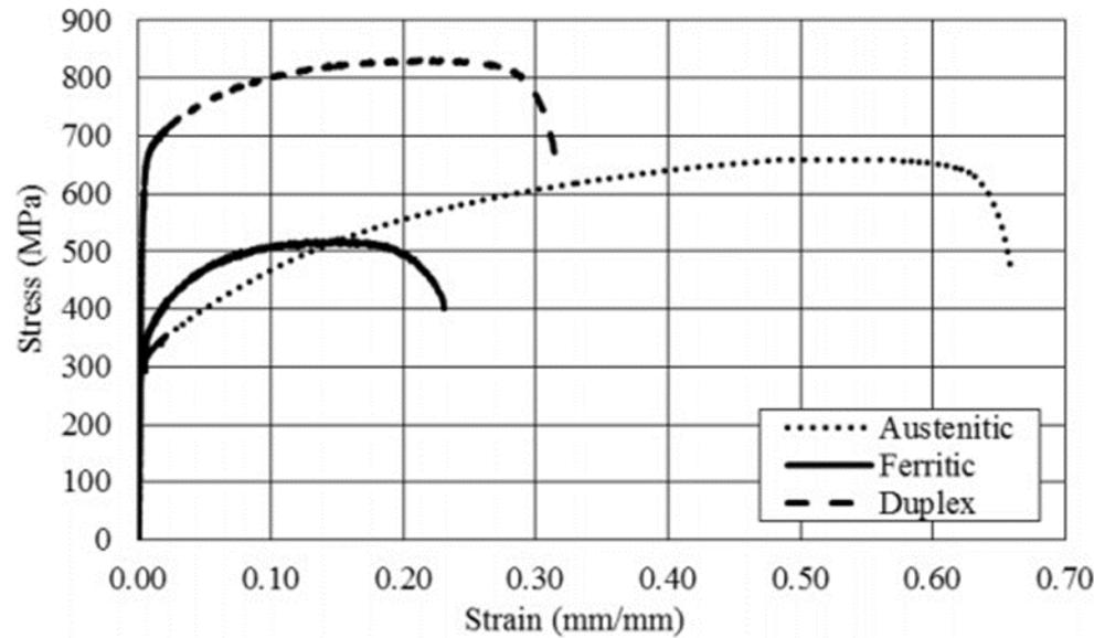
**Figure 1. Stress- strain curves for various types of stainless steels (Arrayago et al., (2015))**
