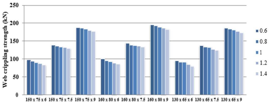
Fig 14. Variation of web crippling strength with inside bend radius for 600 mm samples
