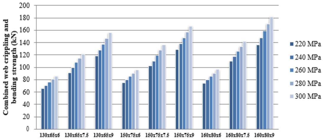
Fig 12. Variation of combined web crippling and bending strength with yield Strength 1000 mm sample
