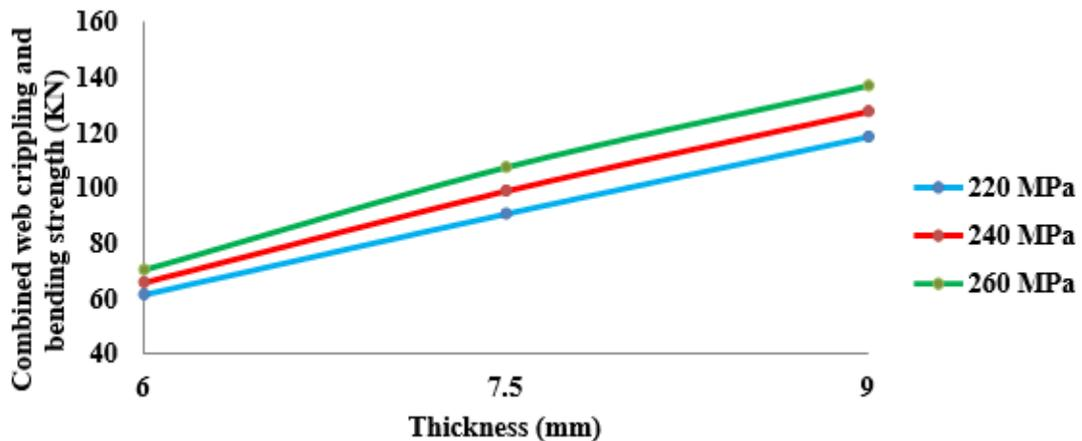
Fig 19. Variation of combined web crippling and bending strength with thickness for 130x65 sample
