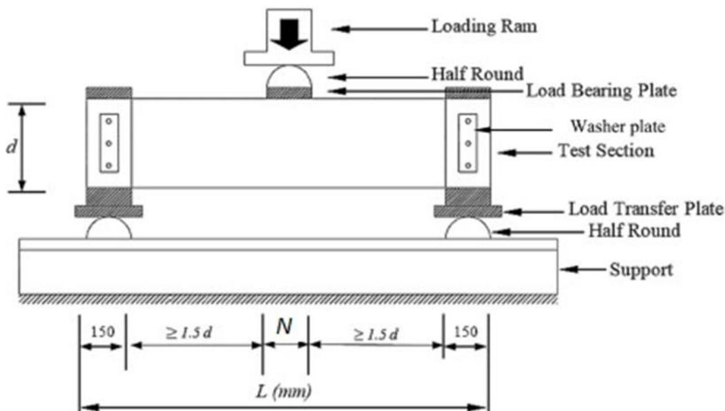
Fig 2. Front view of test setup
