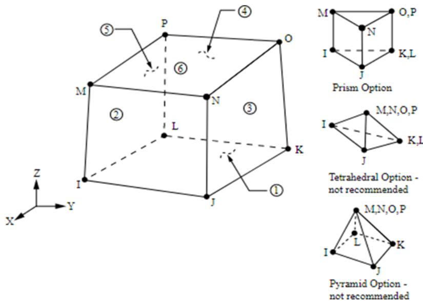
Fig 5. SOLID185 geometry
