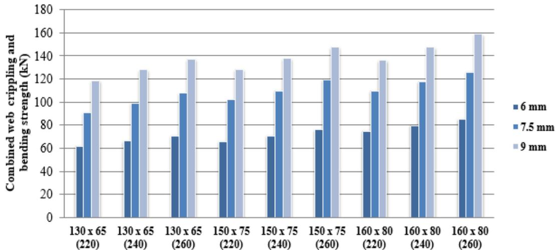
**Fig 20. Variation of combined web crippling and bending strength with thickness for 1000 mm samples**
