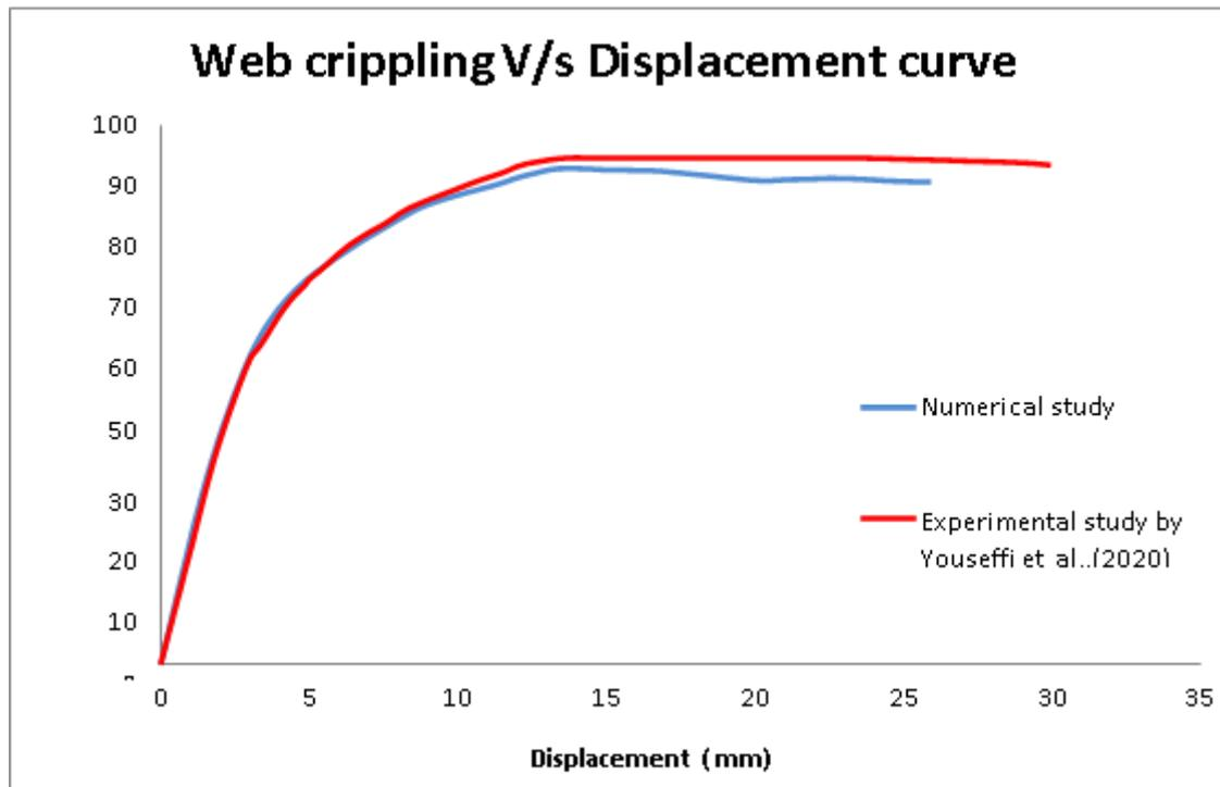
**Fig 8. Web crippling strength V/s displacement comparison**
