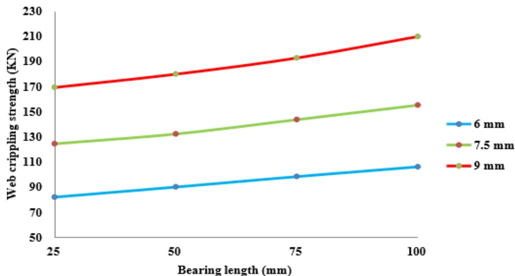
**Fig 21. Variation of web crippling strength with bearing length for 600 mm samples**
