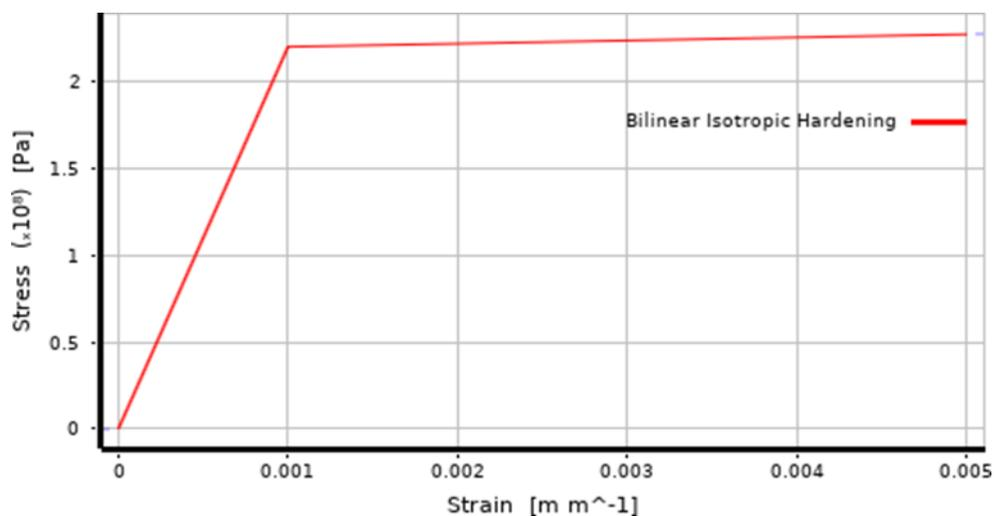
Fig 6. Bilinear stress-strain curve for stainless steel from ANSYS
