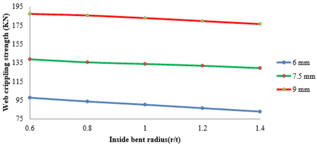
Fig 13. Variation of web crippling strength with inside bend radius for 130x65 sample
