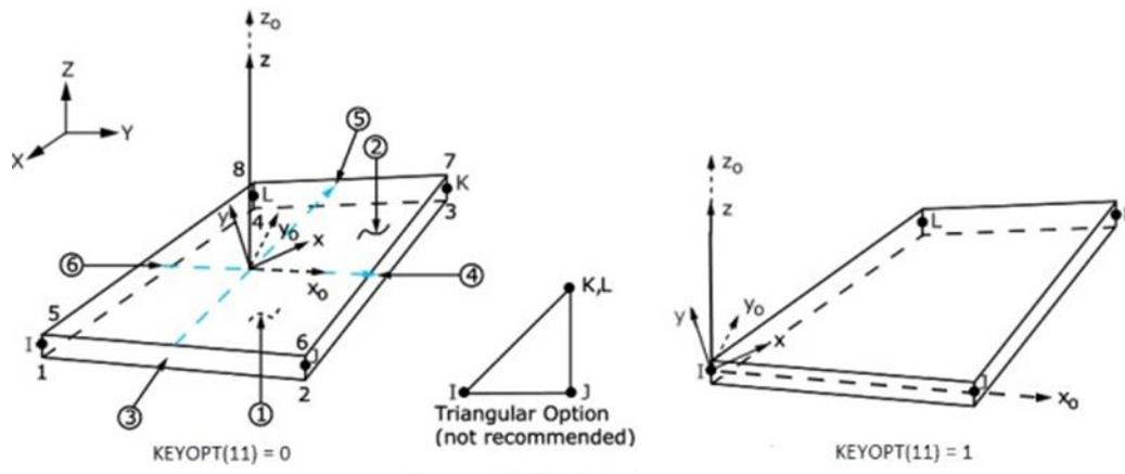
Fig 4. SHELL181 geometry
