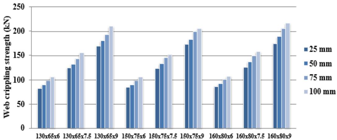
Fig 22. Variation of combined web crippling and bending strength with thickness for 600 mm samples.
