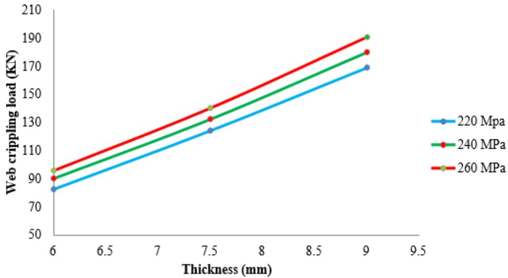
Fig 17. Variation of web crippling strength with thickness for 130x65 sample
