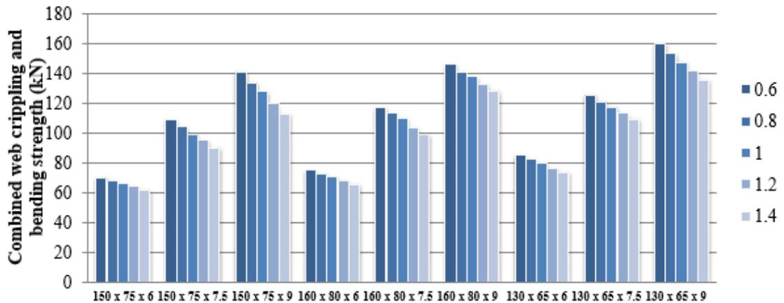
**Fig 16. Variation of combined web crippling and bending strength with inside bend radius for 1000 mm samples**
