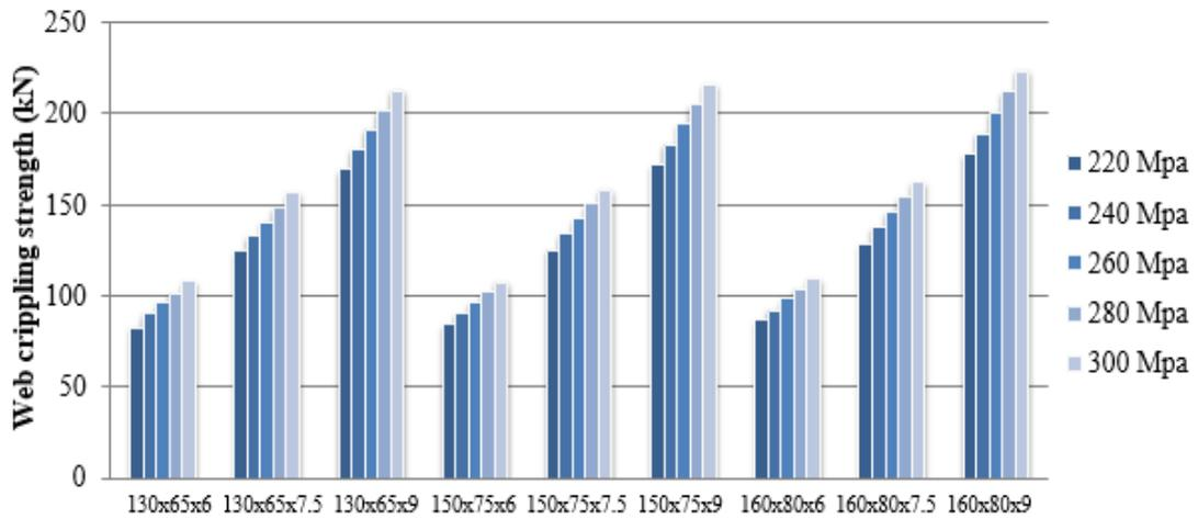
Fig 10 Variation of web crippling strength with yield strength for 600 mm length samples
