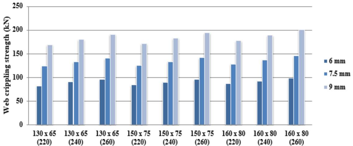
Fig 18. Variation of web crippling strength with thickness radius for 600 mm samples
