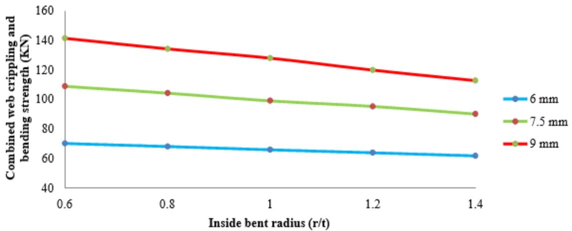
**Fig 15. Variation of combined web crippling and bending strength with inside bend radius for 130x65 sample**
