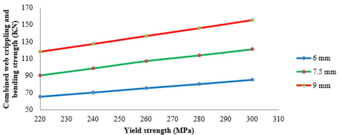
Fig 11. Variation of combined web crippling and bending strength with yield strength 130x65 sample
