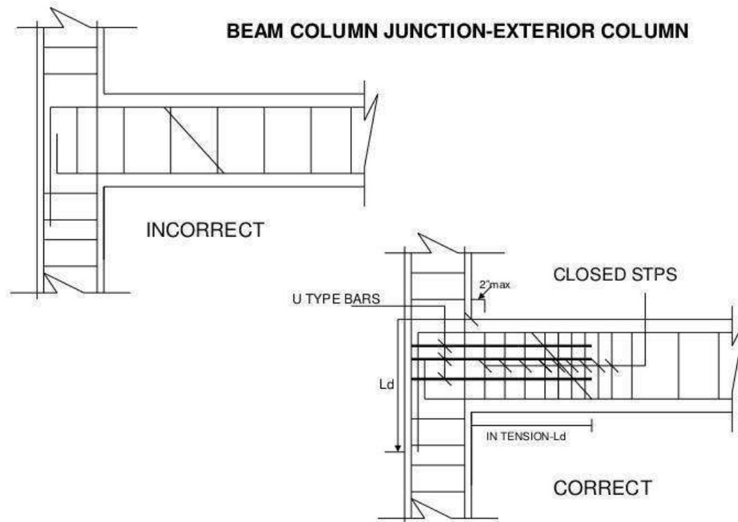
The reversal of stresses during seismic activities makes conservatively designing corner joints as opening joints with the required details necessary.
