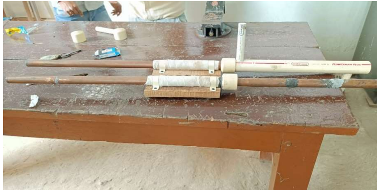
Figure-01 Heat pipe with water jacket with inlet and outlet of condensing section
