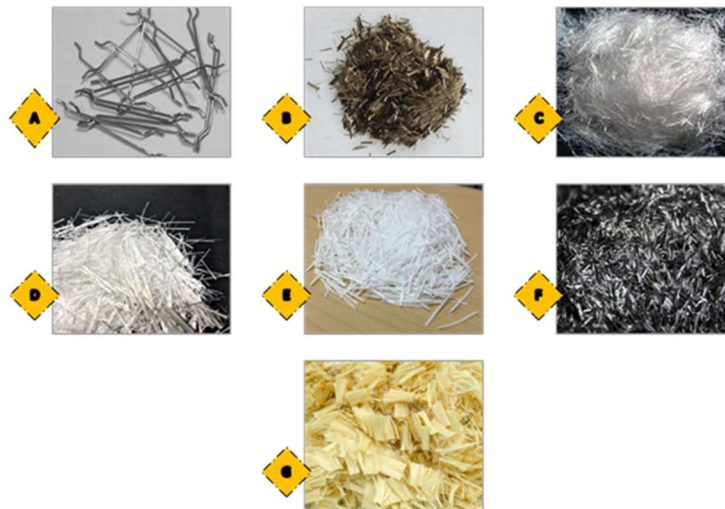
Figure 5: Different types of fibers (a) Steel fibers; (b) Basalt fibers; (c) E-Glass fiber; (d) S-Glass fibers; (e) Polypropylene fibers; (f) Carbon fibers; (g) Aramid fibers
