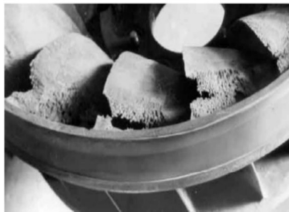
Fig.2. Damage of impeller by cavitation (source: Wu, K. et al., 2019)
