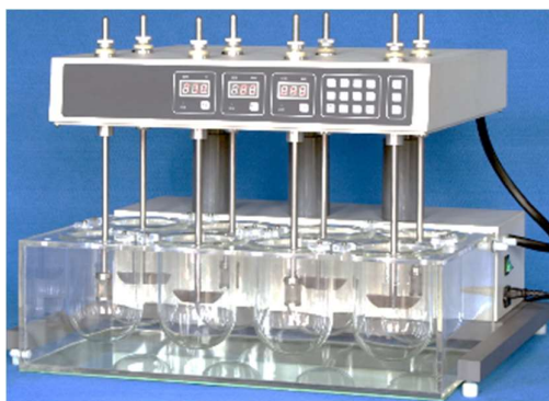
Figure.4 USP Dissolution Apparatus (Paddle Method) for testing drug release from solid dosage forms.
