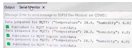
Fig. 3: Serial monitor output displaying JSON-formatted temperature and humidity data published via MQTT.
