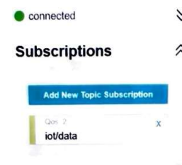
Fig. 4: The HiveMQ WebSocket client is subscribed to the topic iot/data, enabling reception of real-time temperature and humidity data published by the ESP32.
