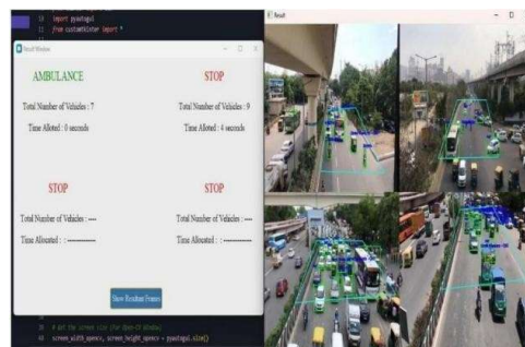
Figure 3. Vehicle detection output and user interface showing ambulance priority.
