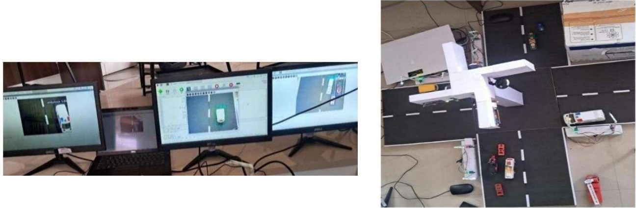
Figure 4. Prototype and testbed setup: (a) multi-monitor system monitoring, (b) physical junction model with sensing and control.
