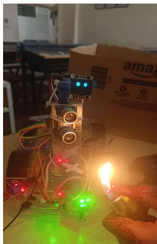
Fig 4: Fire Extinguishing Robo Car Detecting Fire
