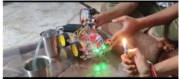
Fig.5: Fire Extinguishing Robo Car Detecting Fire and Sprinkling Water
