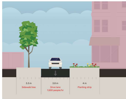
Figure 4: School of Architecture Street Section
