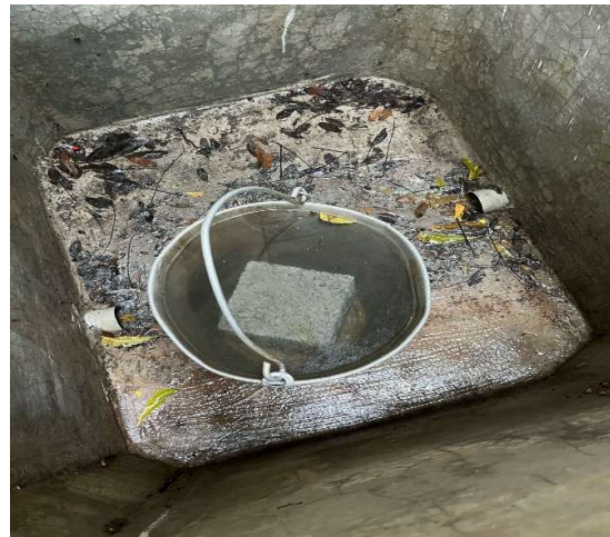
Fig. curing of PET Concrete cube
