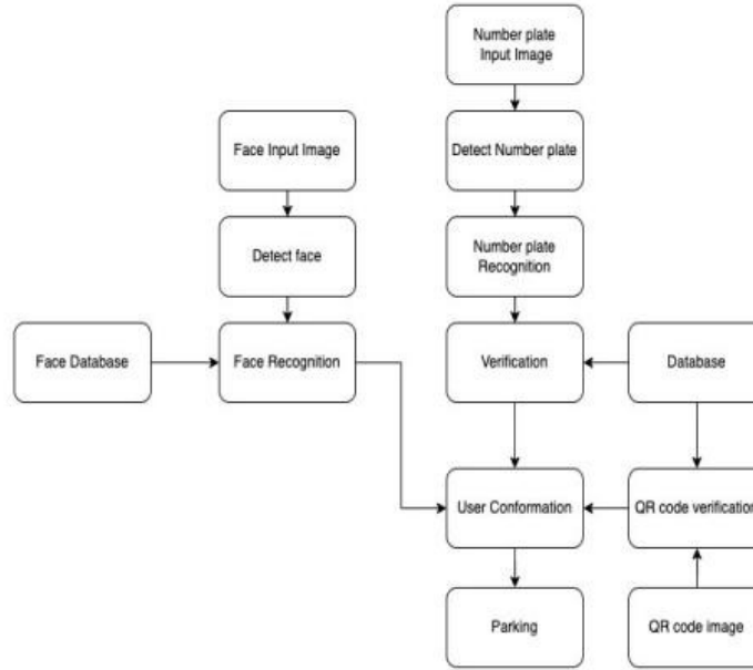
Fig. 1. Block Diagram Representation Triple Authentication For Car Parking
